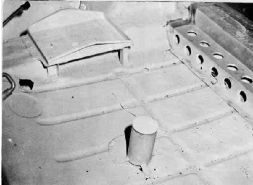
Battery tray, bag tank support and simple post fixing for spare wheel (held down by 2 'bungees').
